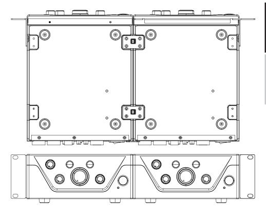
**UNDER-TABLE MOUNTING** (rack-mount bracket included in optionally available rack mounting kit LDIMARK).
