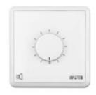
The E-VOL120 is a 100 volt volume control that can handle up to 120 watts of power. It is very versatile thanks to the step-by-step attenuation in 11 steps + zero position. The E-VOL 120 is designed to handle 24V priority signals. This means that you can always get an announcement out, even to zones where the local volume control is in the 'OFF' position!
