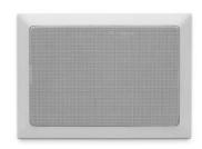
CMR20T is a very compact and performant two-way rectangular 100 volt built-in speaker, provided with a 5.25" polypropylene woofer and 1" tweeter. The two-way aspect makes the loudspeaker very suitable for the reproduction of both background music and microphone calls.
