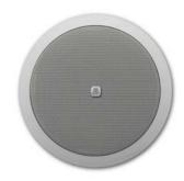
The CM6T is a two-way low impedance or 100 volt loudspeaker suitable for the distribution of microphone calls and background music. In 16 ohms use, you can connect up to 4 loudspeakers in parallel on each channel of a standard 4 ohms amplifier.
