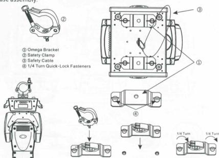
Regardless of the rigging option you choose for your iLED FOX BEAM 90W, always be sure to secure your fixture with a safety cable. The fixture provides a built-in rigging point for a safety cable on the hanging bracket as illustrated above. Be sure to only use the designated rigging point for the safety cable and never secure a safety cable to a carrying handle.
