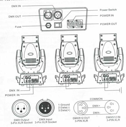
For installations where the DMX cable has to run a long distance or is in an electrically noisy environment, such as in a discotheque, it is recommended to use a DMX terminator. This helps in preventing corruption of the digital control signal by electrical noise. The DMX terminator is simply an XLR plug with a  $120\ \Omega$  resistor connected between pins 2 and 3,which is then plugged into the output XLR socket of the last fixture in the chain. Please see illustrations below.
