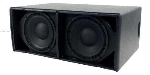
The SX210 is a slimline dual-driver subwoofer designed for situations that call for a visually unobtrusive enclosure. It can be used singly, stacked or flown via integral M8 inserts and its ultra-compact size makes it ideal for applications where space is limited. It features dual 10" (250mm)/2" (50mm) voice coil drivers and generously sized low frequency ports for reduced air noise.
