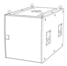
Remove the M10 counter-sunk screws and screw the eyebolts into position. We would recommend four eyebolts and an additional eyebolt as a redundant safety bond. This should be attached to a different point than the other bolts to support the cabinet in the event of the other points failing.
