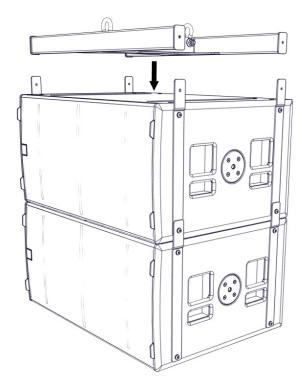
Join using the four M10 x 50 button head screws and washers supplied with the grid assembly. The sub can now be safely flow to the desired height.
