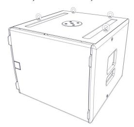
Remove the M10 counter-sunk screws and screw the eyebolts into position. We would recommend four eyebolts and an additional eyebolt as a redundant safety bond. This should be attached to a different point than the other bolts to support the cabinet in the event of the other points failing.
