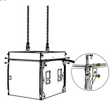
Raise the WPSGRIDt and SXCF118 to a height suitable to fit another SXCF118 below the array, lower it making sure the protective nylon skids line up and fit into the recessed channels on the SXCF118 below.
