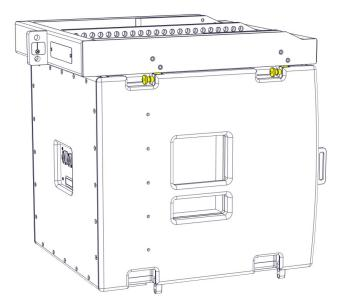
If more subs are to be linked under the first, raise the height of the first sub so you can position a second sub directly under the first. Remove the flying pins in the bottom drop-down rigging links in the first sub and lower it onto the second ensuring that the rigging links engaging all four rigging slots in the second sub exactly as you did with the frame and first cabinet.
