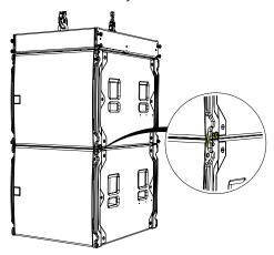
Repeat the procedure for each sub to be included in the array to a maximum of 16 SXCF118. For arrays that consist of SXCF118 and WPS, please refer to the WPS manual.
