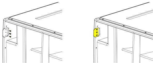
Replace the grill supports and fit the grille making sure the safety screws are used.\
