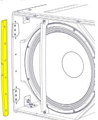
Remove the three screws from the bracket.
