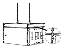
Remove the pins from the stow position, rotate the links to line up with the pin hole position on the SXHF218 above.
