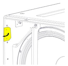
Screw the bracket back in place and repeat for the other three brackets.
