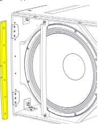
Remove the three screws from the bracket.
