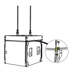
Remove the pins from the stow position, rotate the links to line up with the pin hole position on the SXCF118 above.
