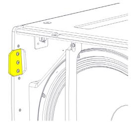
Replace the grill supports and fit the grille making sure the safety screws are used.  $\$
