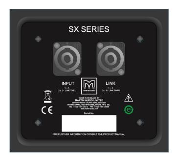
The SX110 has a pair of NL4 connectors on the rear panel. These are wired in parallel and whilst one is nominally labelled 'INPUT' and the other as 'LINK', connection in and out can be made to either connector. Connection to the drive unit(s) is made to pins 1+/-. There is no internal connection to pins 2+/- although these are linked together so can be used for example to carry a mid/top signal and connected to a full range system using a cable wired with reverse connections (pins 2 to pins 1).
