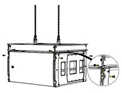
Raise the WPLGRIDt and SXHF218 to a height suitable to fit another SXHF218 below the array, lower it making sure the protective nylon skids line up and fit into the recessed channels on the SXHF218 below.
