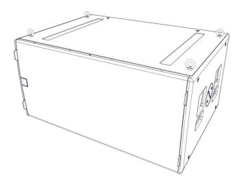
Remove the M10 counter-sunk screws and screw the eyebolts into position. We would recommend four eyebolts and an additional eyebolt as a redundant safety bond. This should be attached to a different point than the other bolts to support the cabinet in the event of the other points failing.
