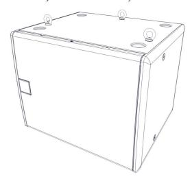
Remove the M10 counter-sunk screws and screw the eyebolts into position. We would recommend three eyebolts and an additional eyebolt as a redundant safety bond. This should be attached to a different point than the other bolts to support the cabinet in the event of the other points failing.
