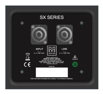
The SX112 has a pair of NL4 connectors on the rear panel. These are wired in parallel and whilst one is nominally labelled 'INPUT' and the other as 'LINK', connection in and out can be made to either connector. Connection to the drive unit(s) is made to pins 1+/-. There is no internal connection to pins 2+/- although these are linked together so can be used for example to carry a mid/top signal and connected to a full range system using a cable wired with reverse connections (pins 2 to pins 1).
