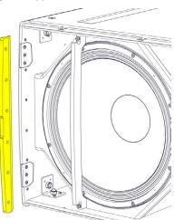
Remove the three screws from the bracket.
