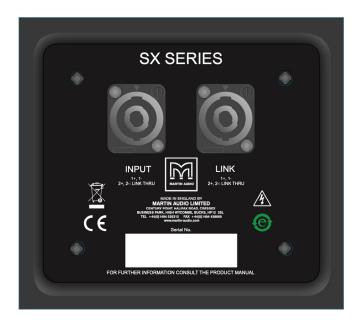
The SXF115 has a pair of NL4 connectors on the rear panel. These are wired in parallel and whilst one is nominally labelled 'INPUT' and the other as 'LINK', connection in and out can be made to either connector. Connection to the drive unit(s) is made to pins 1+/-. There is no internal connection to pins 2+/- although these are linked together so can be used for example to carry a mid/top signal and connected to a full range system using a cable wired with reverse connections (pins 2 to pins 1).
