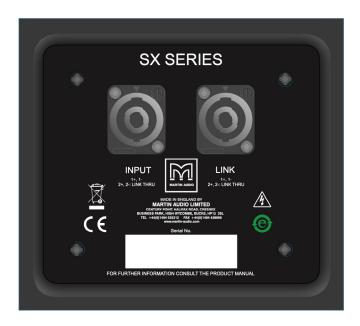
The SX118 has a pair of NL4 connectors on the rear panel. These are wired in parallel and whilst one is nominally labelled 'INPUT' and the other as 'LINK', connection in and out can be made to either connector. Connection to the drive unit(s) is made to pins 1+/-. There is no internal connection to pins 2+/- although these are linked together so can be used for example to carry a mid/top signal and connected to a full range system using a cable wired with reverse connections (pins 2 to pins 1).
