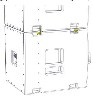
More cabinets can be added as required or transition frames connected to enable flying of either MLA Mini or WPM arrays under the SXP115. For more details see the User Guides for MLA Mini and WPM.
