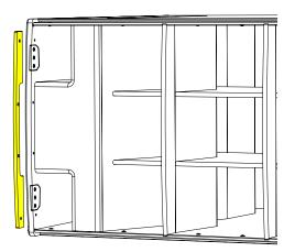
Remove the three screws from the bracket.
