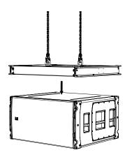
Replace the WPLGRIDt pins to link the SXHF218 securely to the WPLGRIDt. The SXHF218 pins for the first cabinet are not needed in this configuration and can be placed back in the stowed position.
