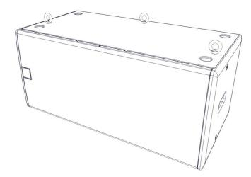
Remove the M10 counter-sunk screws and screw the eyebolts into position. We would recommend three eyebolts and an additional eyebolt as a redundant safety bond. This should be attached to a different point than the other bolts to support the cabinet in the event of the other points failing.
