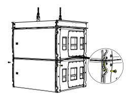
Remove the 4 link pins from the WPLGRIDt and also remove the 4 pins from the from SXHF218 to release the links. Rotate the SXHF218 links and line them up with the pin holes in the WPLGRIDt.
