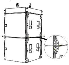
Remove the pins from the from SXCF118 to release the links. Rotate the SXCF118 links and line them up with the pin holes in the WPSGRIDt.
