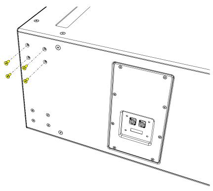
Position each castor over the insets and screw into place using the fixings supplied in the kit.
