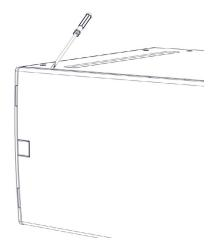
Remove the screws from the grille support on the side of the cabinet and remove the grille support.
