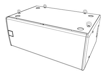
Remove the M8 counter-sunk screws and screw the eyebolts into position. We would recommend four eyebolts and an additional eyebolt as a redundant safety bond. This should be attached to a different point than the other bolts to support the cabinet in the event of the other points failing.
