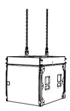
Replace the pins to link and lock the SXCF118 securely to the WPSGRIDt.
