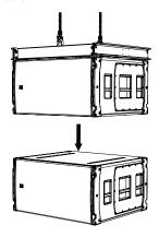
Replace the pins into the lock position on the cabinet above making sure all four links are securely attached. Repeat the process until the correct amount of SXHF218's are flown, the maximum number is 16 SXHF218.
