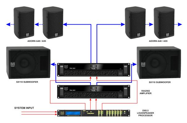
System 4 - Using a 4-channel VIA amplifier
