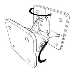
The first stage is to disassemble the bracket so that the cabinet half can be fitted to the speaker and the wall section attached to the wall. A 4mm allen key is required. If adjustment is only required in one plane, vertical or horizontal, the middle section can be removed. This has the added advantage that the speaker will be closer to the wall.
