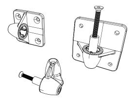
Fit the wall bracket in the appropriate orientation for horizontal or vertical adjustment. Fixings appropriate for the wall surface and weight of the cabinet must be used to ensure a safe and secure installation.
